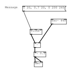
Use this one to play A440 with an envelope. The envelope ramps up to amplitude 1 in 20 ms, then down to 0.7 in another 20 ms, then sustains for 260 ms and then ramps down to 0 in 200 ms. So the total envelope time is 500 ms. Edit the times to change the envelope or edit the frequency 440 to change the pitch.
